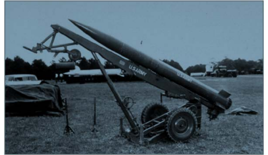
Figure 64 LITTLE JOHN short-range rocket
